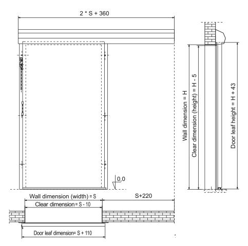
Sliding chiller doors - classical sliding system, angle frame.
